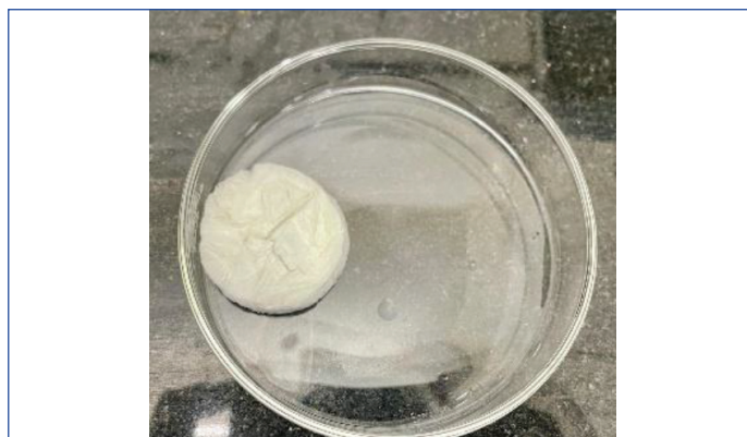
[Table/Fig-2]: Chitosan-Zinc Oxide mixture cast into sterile petri-dishes to obtain a porous CS-ZnO scaffold.
