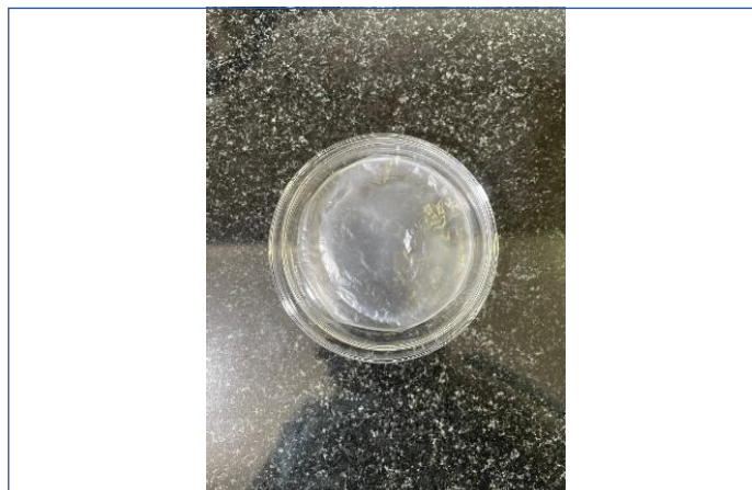
[Table/Fig-3]: Uniform PCL film after complete solvent evaporation.
