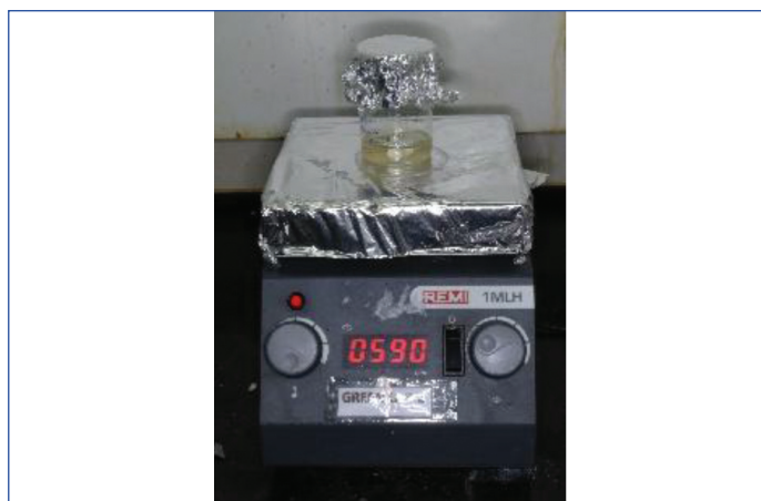
[Table/Fig-1]: Sodium hydroxide (NaOH) and Zinc Nitrate hexahydrate \{Zn(NO_3)_2 \cdot 6H_2O\} solution under continuous magnetic stirring.
