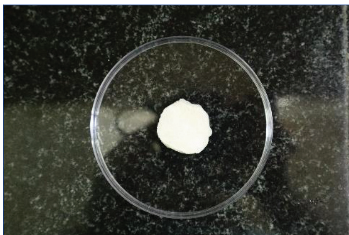
[Table/Fig-4]: Bilayered scaffold obtained after complete chloroform evaporation.
